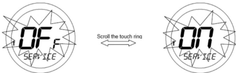
If you require **SERVICE** mode activated, use the touch ring to scroll from **OFF** to **ON** and press **OK**.
