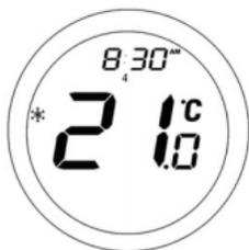
If the ST620 is operating in FROST mode the LCD will not indicate MANUAL or AUTO, but will display both the room temperature and also the FROST mode indicator.
