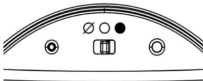
2. Gently press and hold the SYNC button with a blunt object. After 3 seconds the Boiler Control LED will flash once every second to indicate it is ready to pair and ready to receive a signal from the ST620. The Boiler Control will remain in pairing mode for 12 minutes.
