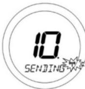
The display counts down for a period of 10 minutes, with the RF Signal indicator flashing while the signal is being transmitted. The RF address code will be generated randomly.
