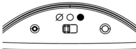
8. To ensure the boiler control is connected properly, please now move the switch to ON
