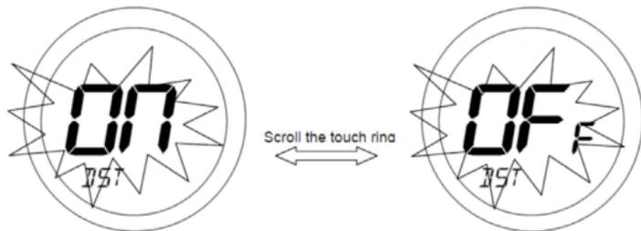
Use the Touch Ring to scroll to set the DST option ON or OFF, and confirm the setting using the OK button – the default setting is ON. Press the Arrow key to return to the previous screen display, or do nothing for 10 seconds and the ST620 will return to NORMAL mode.
