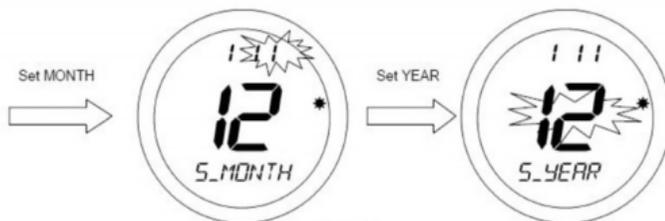
After confirming the year setting by pressing the OK key, the display will then change to display the first screen for entering the holiday end date.
