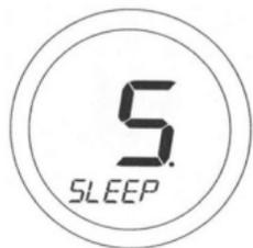
Pressing the Touch Ring for 1 second will turn on the LCD backlight, and pressing the Touch Ring for 3 seconds will wake the ST620 from SLEEP mode and restore the programmable thermostat to AUTO mode.
