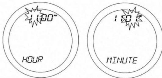
Use the Touch Ring to scroll to set the hour and confirm the choice using the OK button. The minute setting will then be selected – change this setting in the same way using the Touch Ring, and confirm the setting using the OK button. After setting the time, the next screen display allows you to set the date – this is set in exactly the same way as previously described for the time.
