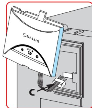
5. Now locate the boiler control's four hooks then press in and down. Replace Cover panel A.
