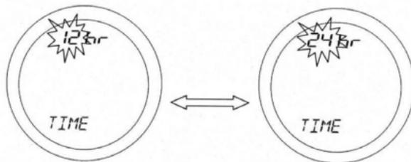
On entering the menu, use the Touch Ring to scroll to the preferred option (12 or 24 hour clock), and confirm the choice using the OK button. Use the Arrow key to return to the previous screen display. After setting the time display format, the next screen display allows you to set the time.
