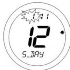
The month setting ('S\_MONTH') will then be selected – change this setting in the same way using the Touch Ring, and confirm the setting using the OK button. Finally, set the year ('S\_YEAR') – this is done in exactly the same way as previously described for the date and month.
