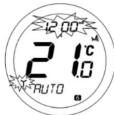
The RCC status indicator will be displayed for 10 minutes during clock updates. The indicator will flash during the time update process, after which the indicator will be displayed for 5 minutes before turning off.
