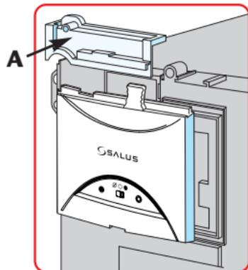
6. Replace the front fascia and boiler's outer casing
