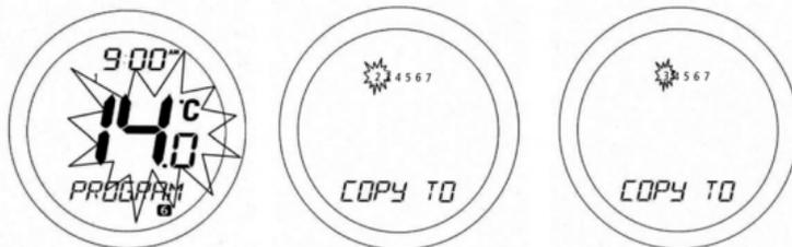
After entering the settings in Programmes 1 to 6 for Monday(1), the ST620 display will change to display a COPY TO screen. On this screen, scroll to the day that you want to copy the settings to using the Touch Ring, and then confirm this by pressing the OK key. The ST620 will then move to the next day and ask if you would like to copy again.
