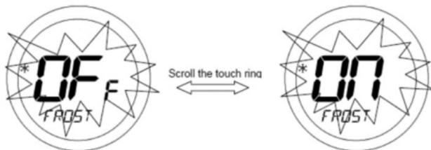
On entering the menu, use the Touch Ring to scroll to the preferred option (OFF or ON), and confirm the choice using the OK button. Use the Arrow key to return to the Menu Option display.
